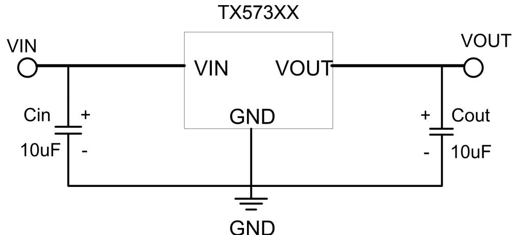
Note1:  $C_{in}=C_{out}=10\mu F$ . (10uF Electrolytic capacitor is recommended).
